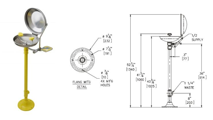
Model S0340-CS1 is our free standing eye wash with lid and stainless steel bowl. Complete with yellow plastic spray heads, chrome plated brass stay open ball valve and stainless steel clamshell cover. Push handle operated.
